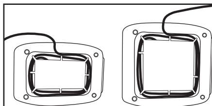
Shorten cord, if necessary, by wrapping cord under the base. The Toaster's feet are tall enough to allow the cord to exit from under any side of the Toaster.
