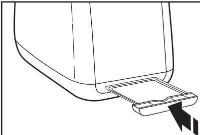
**4** Return crumb tray to Toaster. Press it in firmly until it clicks into position. Do not use the Toaster without the crumb tray in proper position.
