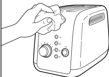
**3** Wipe Toaster with a soft, damp cotton cloth. Do not use paper towels, abrasive cleansers or liquid cleaning products. Do not immerse Toaster in water.
